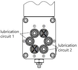
Linear unit 1 Lubrication circuit 1
